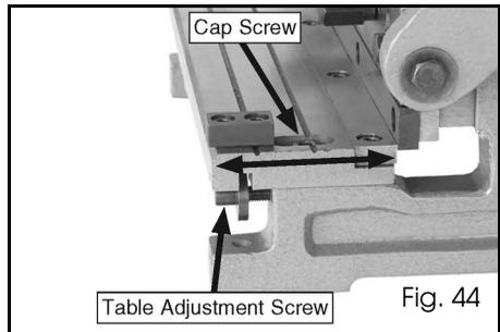
**NOTE:** Rotating the table adjustment screws clockwise moves the table toward the upper shear blade.
