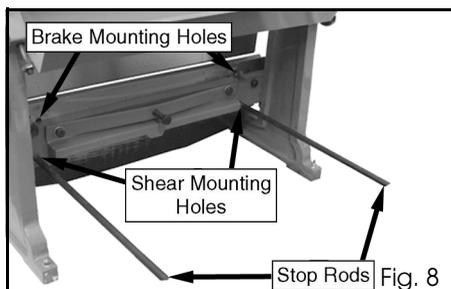
6. Loosen the hex bolts on the stop bar and slide it onto the rods.
