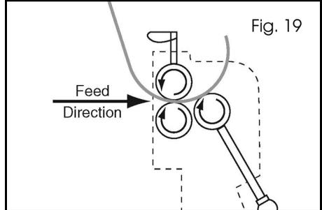
7. Reduce the radius of the curve by raising the rear roller, then repeat Steps 4-7 until you have produced the desired cylinder (see the illustration in Figure 20).
