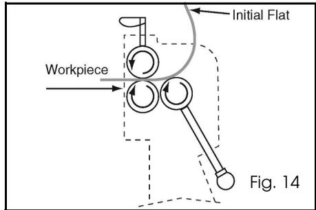
**NOTE:** To make a cone, tighten one adjustment knob more than the other.
